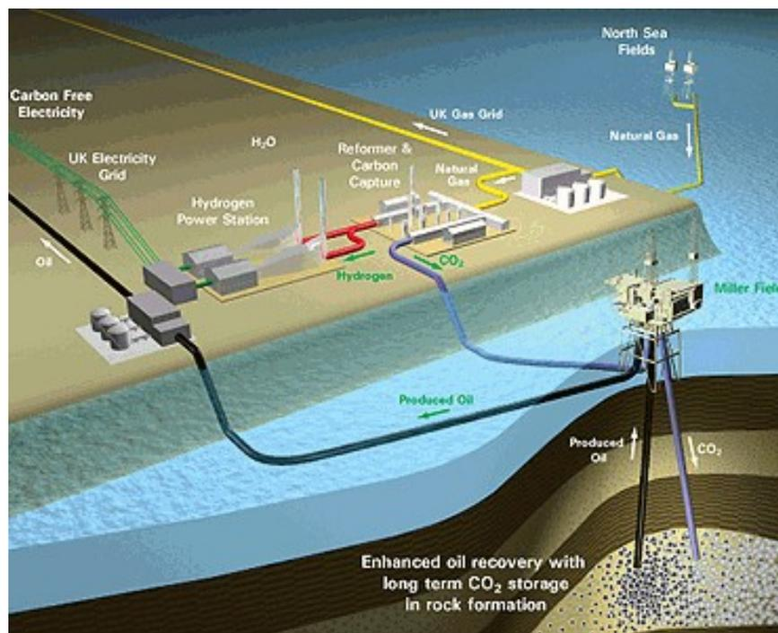
Figure 8 Peterhead Hydrogen Generation with CCS scheme
